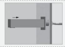
Secure the rosette into position using the anti rotation pin.
