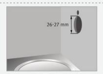
Remove the gasket, the disk, the nut and the flexible pipe from the base of the faucet and insert the faucet through the wall.
