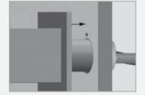
Fix the base behind the wall with the hexagonal nut and the disk.
