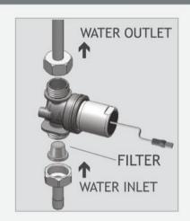
NOTE: Make sure the filter is located between the solenoid housing and the water inlet.
